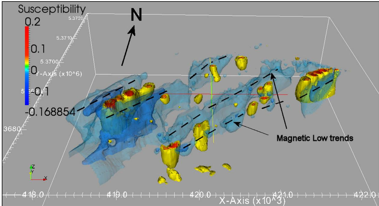
Fault Anomaly Inversion Model – Elevated view from South – Red Isosurface = 0.07 SI, Orange Isosurface = 0.05 SI, Yellow Isosurface = 0.03 SI, Light Blue Isosurface = -0.014 SI, Dark Blue Isosurface = -0.03 SI
