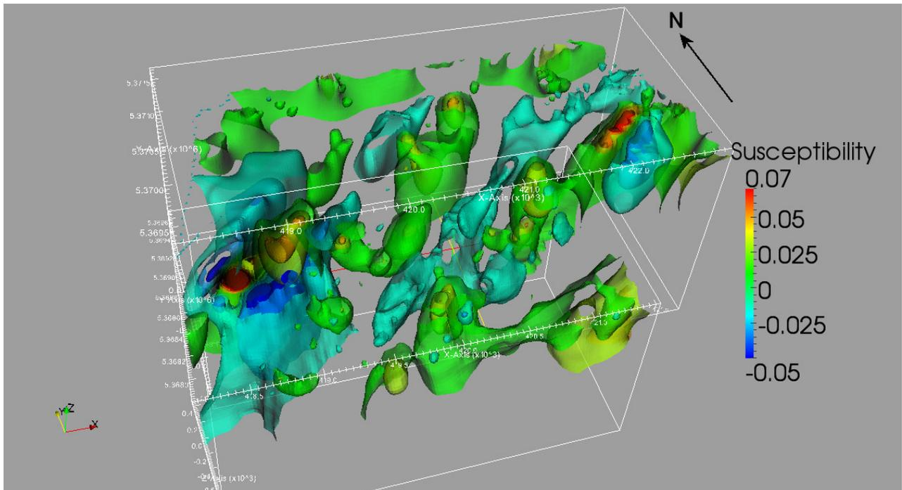
Fault Anomaly Merged North and South Inversion Models – Elevated view from South – Red Isosurface = 0.07 SI, Orange Isosurface = 0.05 SI, Yellow Isosurface = 0.03 SI, Green Isosurface = 0.01 SI, Light Blue Isosurface = -0.014 SI, Blue Isosurface = -0.03 SI, Dark Blue Isosurface = -0.05 SI
