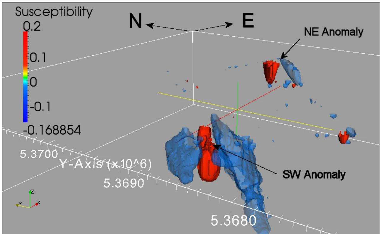
Fault Anomaly Inversion Model – Elevated side view from SW – Red Isosurface = 0.07 SI, Blue Isosurface = -0.03 SI
