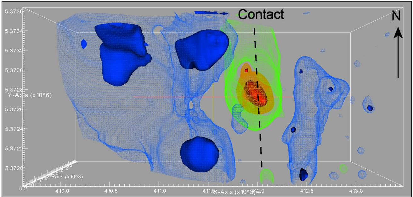
Bulls Eye 3D Inversion Model – Top view – Red Isosurface = 0.07 SI, Orange Mesh Isosurface = 0.05 SI, Green Mesh Isosurface = 0.025 SI, Blue Mesh Isosurface = -0.01 SI, Blue Isosurface = -0.02 SI
