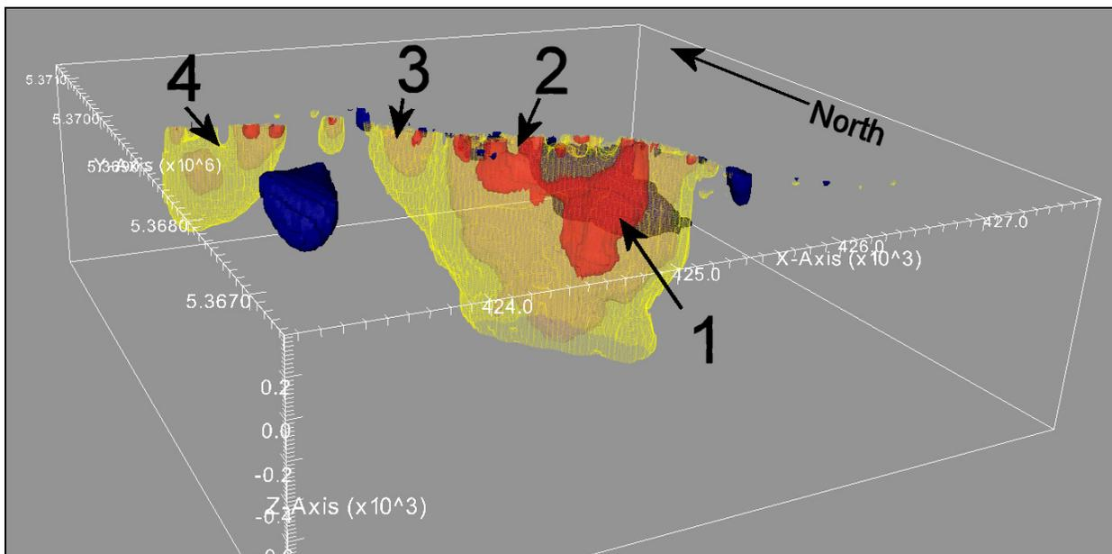
3D Inversion Model – Elevated View from South West – Red Isosurface = 0.26 SI – Pink Mesh Isosurface = 0.19 SI – Yellow Mesh isosurface = 0.15 SI - Blue Isosurface = -0.01 SI. High susceptibility plate extends to greater depth at the Southeast end.
