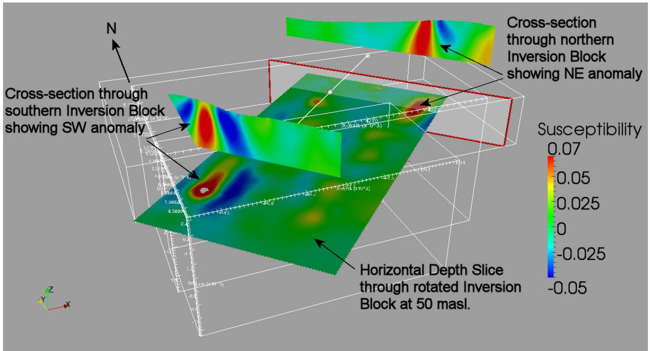
Depth Slice through rotated inversion model. Cross-section through north and south inversion blocks show vertical dip of strong magnetic anomalies and SE dip of flanking low susceptibility bodies.
