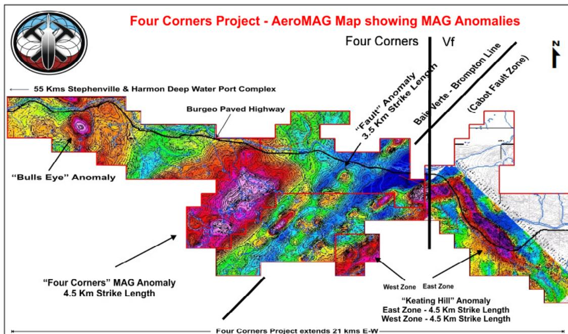
Total Magnetic Field Intensity Colour Contour Maps – based on Fugro airborne survey (Vf block) and Geotech airborne survey (Four Corners block).
