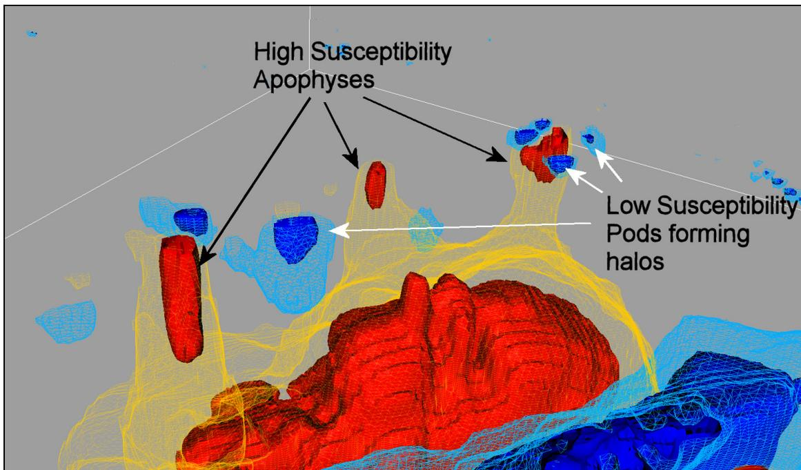
3D Inversion Model – Side View from SE – Red Isosurface = 0.07 SI, Orange mesh isosurface = 0.05 SI, Blue Mesh Isosurface = -0.03 SI, Blue Isosurface = -0.03 SI. Shows high susceptibility apophyses extending up from deep source to surface as near vertical pipes and low susceptibility halos.
