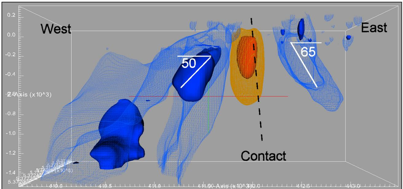
Bulls Eye 3D Inversion Model – Side view from South – Red Isosurface = 0.07 SI, Orange Mesh Isosurface = 0.05 SI, Blue Mesh Isosurface = -0.01 SI, Blue Isosurface = -0.02 SI
