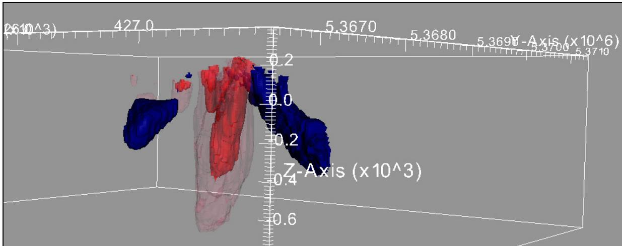
3D Inversion Model – Side View from South East – Red Isosurface = 0.26 SI – Pink Mesh Isosurface = 0.19 SI – Blue Isosurface = -0.01 SI. High susceptibility plate dips  $\sim 80^{\circ}$  SW. Low susceptibility plate dips  $\sim 60^{\circ}$  NE.
