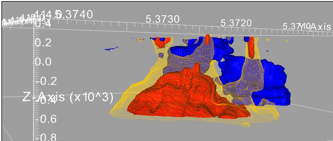
3D Inversion Model – Side View from NW – Red Isosurface = 0.07 SI, Orange mesh isosurface = 0.05 SI. Blue Isosurface = -0.03 SI. Shows high susceptibility apophyses extending up from deep source to surface as near vertical pipes.
