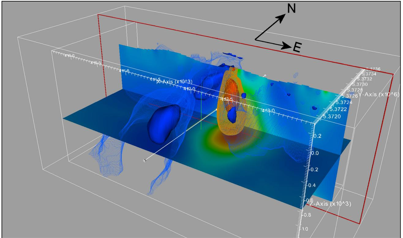
Bulls Eye 3D Inversion Model – Elevated view from South East– Red Isosurface = 0.07 SI, Orange Mesh Isosurface = 0.05 SI, Blue Mesh Isosurface = -0.01 SI, Blue Isosurface = -0.02 SI – Horizontal Slice through model at 1000m depth – Vertical Slice through north end of model
