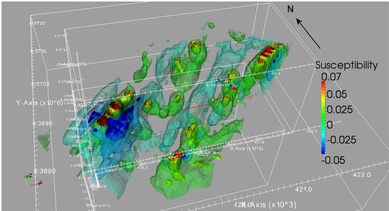
Fault Anomaly Angle Inversion Model – Elevated view from South – Red Isosurface = 0.07 SI, Orange Isosurface = 0.05 SI, Yellow Isosurface = 0.03 SI, Green Isosurface = 0.01 SI, Light Blue Isosurface = -0.014 SI, Blue Isosurface = -0.03 SI, Dark Blue Isosurface = -0.05 SI
