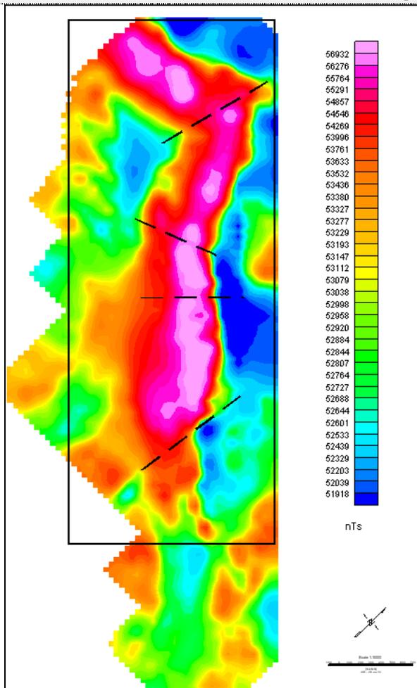
Total magnetic field intensity – VF survey – rotated 45<sup>0</sup> clockwise. Inversion window outlined in black. Possible faults drawn in dashed lines
