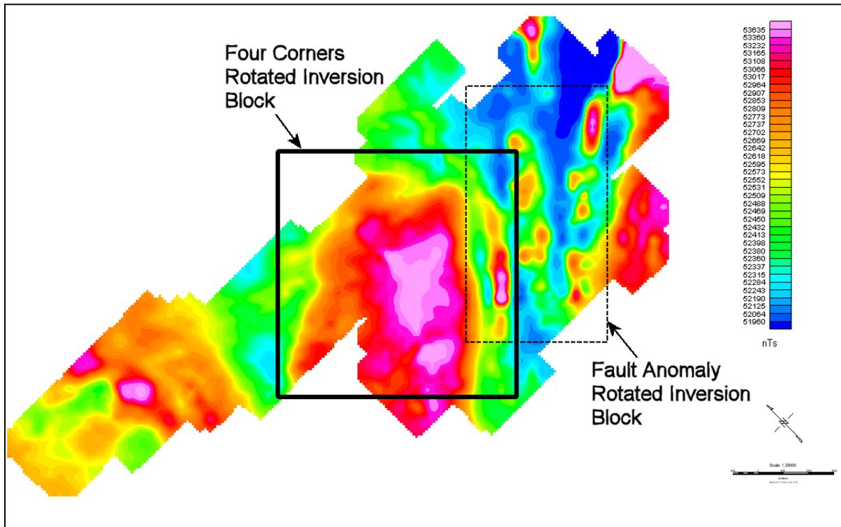
Total Magnetic Field Intensity Colour Contour Map of Geotech Survey – rotated 45<sup>0</sup> counter clockwise
