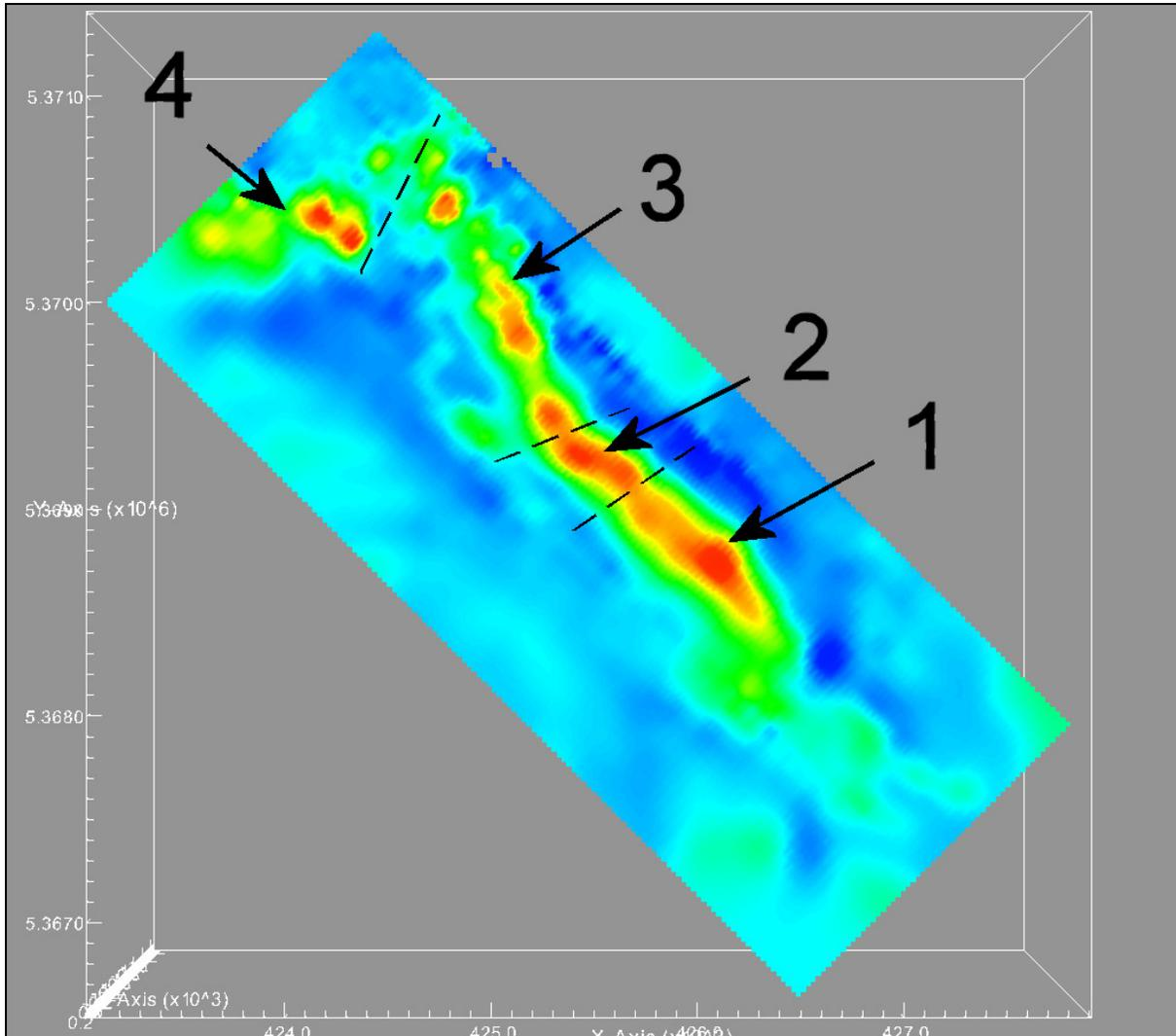
3D Inversion Model – Top View of horizontal depth slice at 75m depth. – NW striking plate can be divided into 4 segments.
