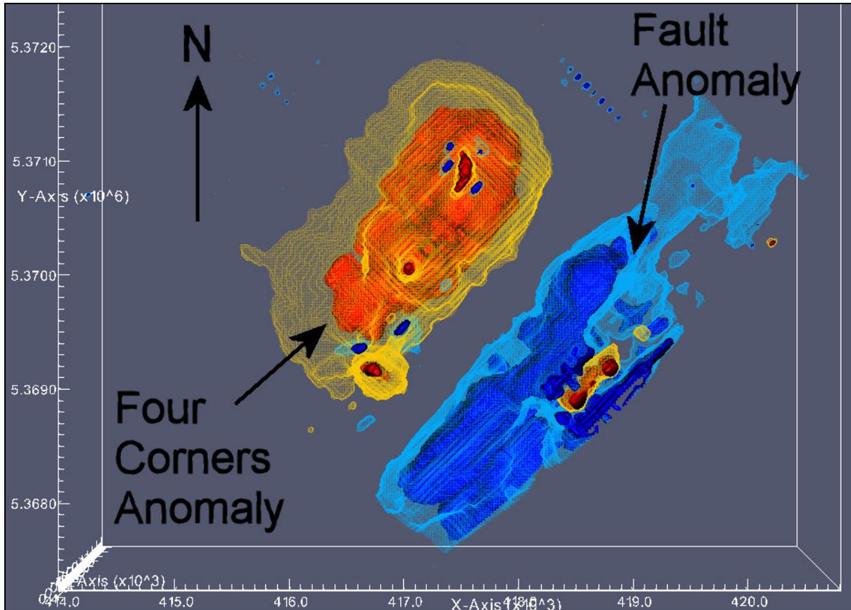
3D Inversion Model – Top View – Red Isosurface = 0.07 SI, Orange mesh isosurface = 0.05 SI. Blue Mesh Isosurface = -0.03 SI, Blue Isosurface = -0.03 SI.
