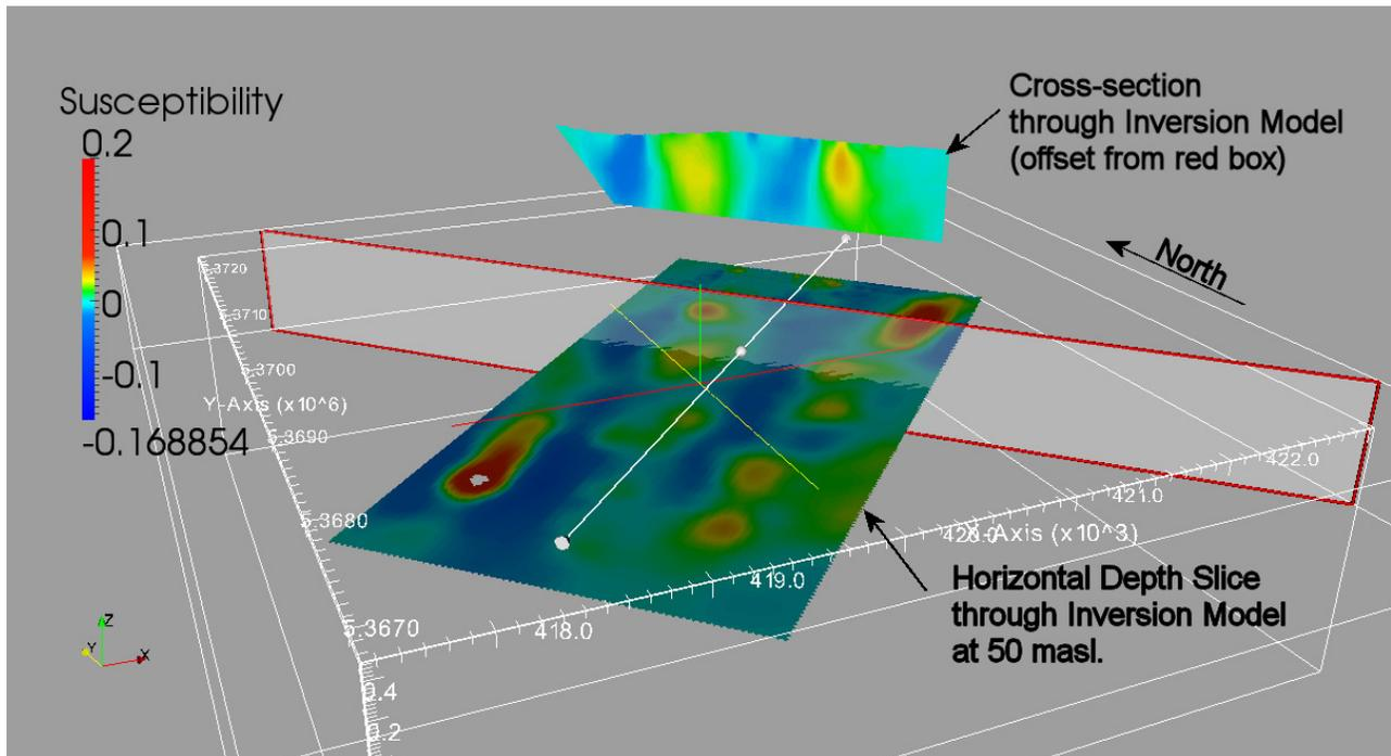
Depth Slice through rotated inversion model. Cross-section through rotated inversion model shows near vertical to steep SE dip of weak magnetic high trends.
