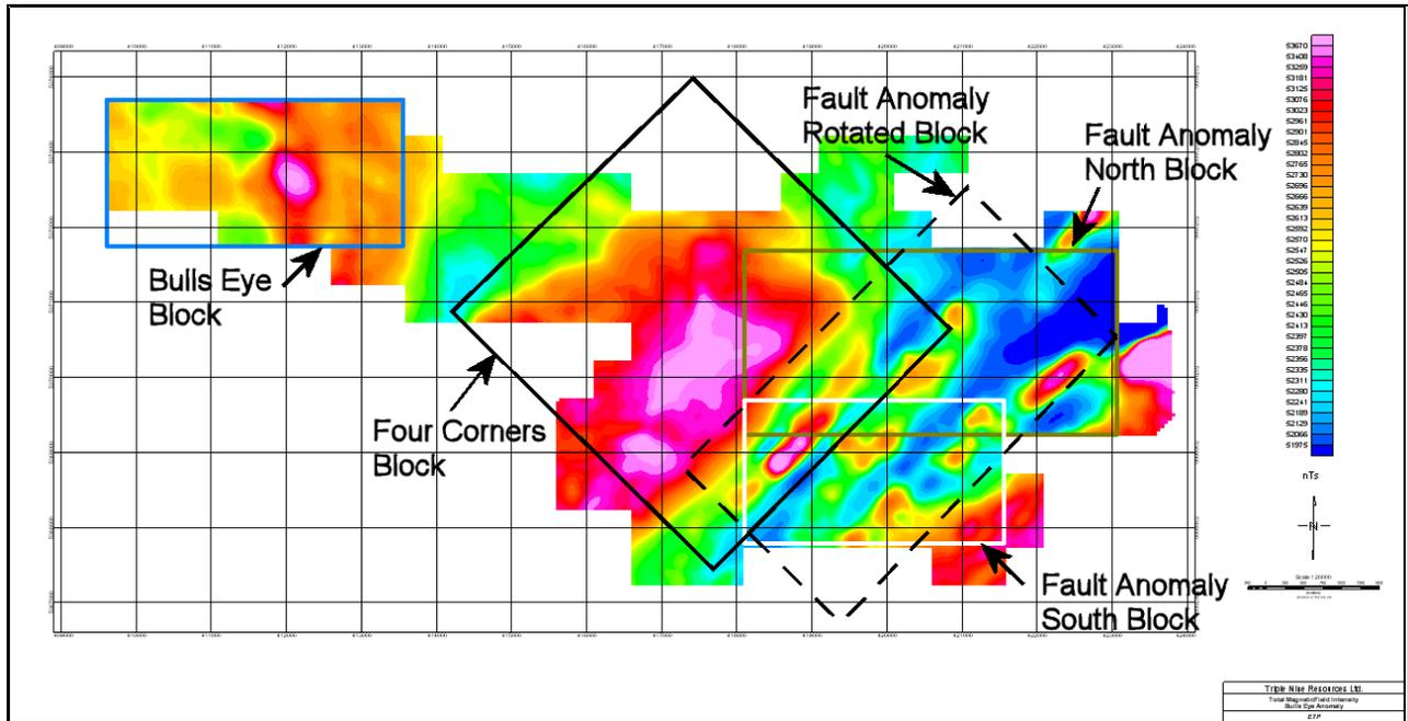
Geotech Airborne Magnetic Survey – Outlines of magnetic data extracted for 3D inversion modelling.
