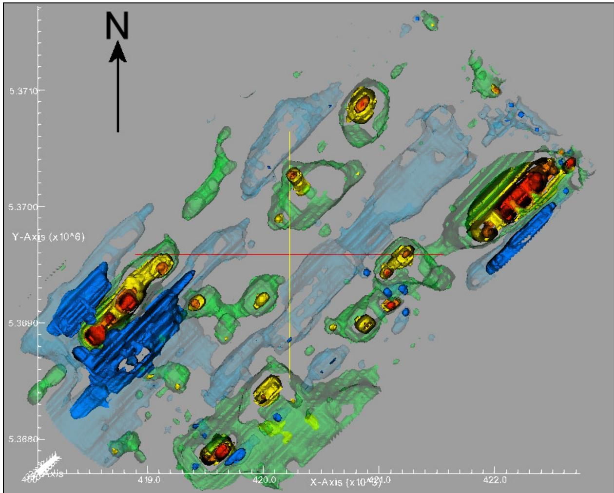
Fault Anomaly Inversion Model – Top View – Red Isosurface = 0.07 SI, Orange Isosurface = 0.05 SI, Yellow Isosurface = 0.03 SI, Green Isosurface = 0.01 SI, Light Blue Isosurface = -0.014 SI, Dark Blue Isosurface = -0.03 SI
