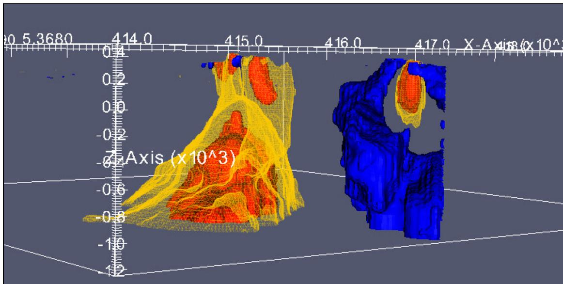
3D Inversion Model – Side View from SW – Red Isosurface = 0.07 SI, Orange mesh isosurface = 0.05 SI. Blue Mesh Isosurface = -0.03 SI, Blue Isosurface = -0.03 SI. Highlights near vertical SE edge and dipping NW edge. Low susceptibility body to the SE maps the western edge of the Fault Anomaly response.
